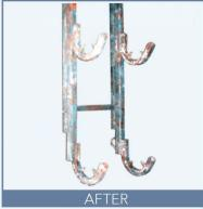
Recognized as the industry leader in thermal stripping and parts reclamation, PCPC Cleaning Ovens safely remove paints, epoxies, powder coating, and other combustibles from paint hangers, racks, hooks and other metal parts. They are fully automatic and self-adjusting – simply load your parts, set your cycle time and the furnace does the work. Plus, its powerful afterburner eliminates all hydrocarbon emissions making them virtually pollution free.
