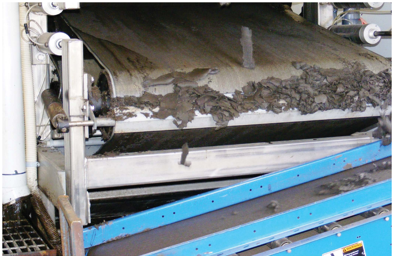
BFP Cake Discharge 6" stands for - "Belt Filter Press, biosolids cake.
