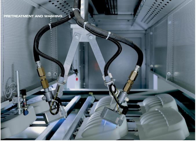
PPG X-BOND Pretreatment is a zirconium-based, thin-film pretreatment system that prepares steel, galvanized steel and aluminum substrates for paint adhesion. With performance equivalent to that of iron phosphates, it provides corrosion resistance and is compatible with low application temperatures.
