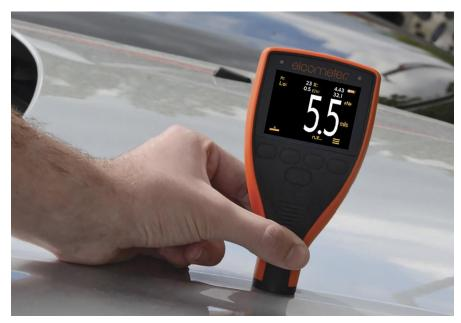
An Elcometer model 3l1 being used to check a car's paint finish.
