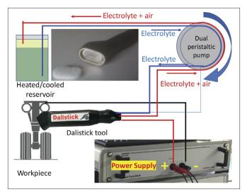
Figure 2: Non-drip selective plating system and closed-loop circuit.
