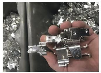
TECHNIBRITE SN 200 tin process provides lustrous, bright tin deposits. Photo Credit: Industrial Plating, Inc.
