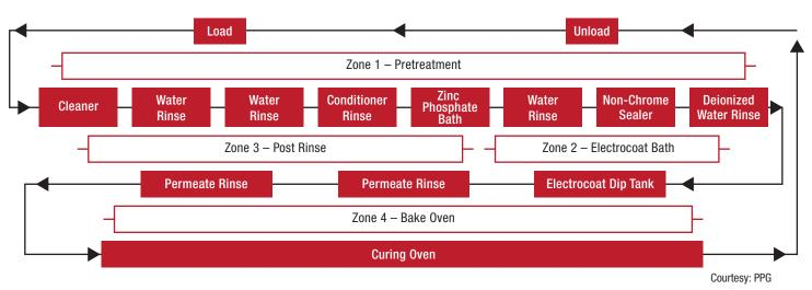
Another key advantage of e-coat is the electrical deposition method itself, ClearClad says. The application of electricity causes the resins and other ingredients to deposit onto the parts' surface. Controlling the electrical current enables a predictable and consistent thickness of coating to be applied. "This is essential if tinted coatings are required such as brass or gold colors over bright nickel or zamak," where consistent color effect demands consistent thickness, the company adds.
