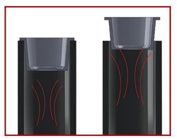
Graphic demonstrating plug blowing out due to pressure buildup.
