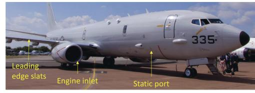
Figure 1: P-8 Poseidon showing areas with bare aluminum subject to corrosion.
