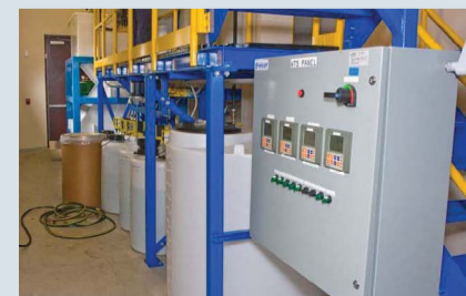
TechCenter waste treatment system, capable of modelling customer waste streams and conducting tests of treatment solutions in a controlled environment.
