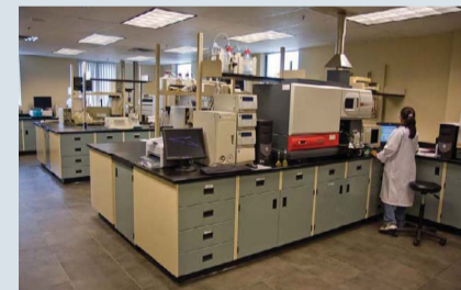
Analytical Instrumentation Lab: Inductively Coupled Plasma Optical Emission Spectrometer (right), multi-metal detection in bath and wastewater solutions.
