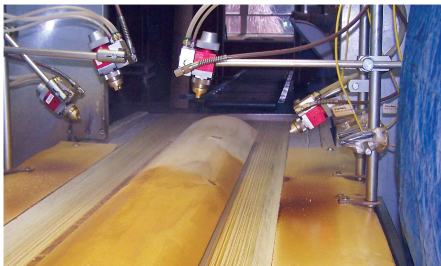
Pine River Inc. located in Charlevoix MI. manufactures log siding systems for the log home industry. Pine River applies two coats of 100 per cent solid UV stain, providing an environmentally sound base coat.
