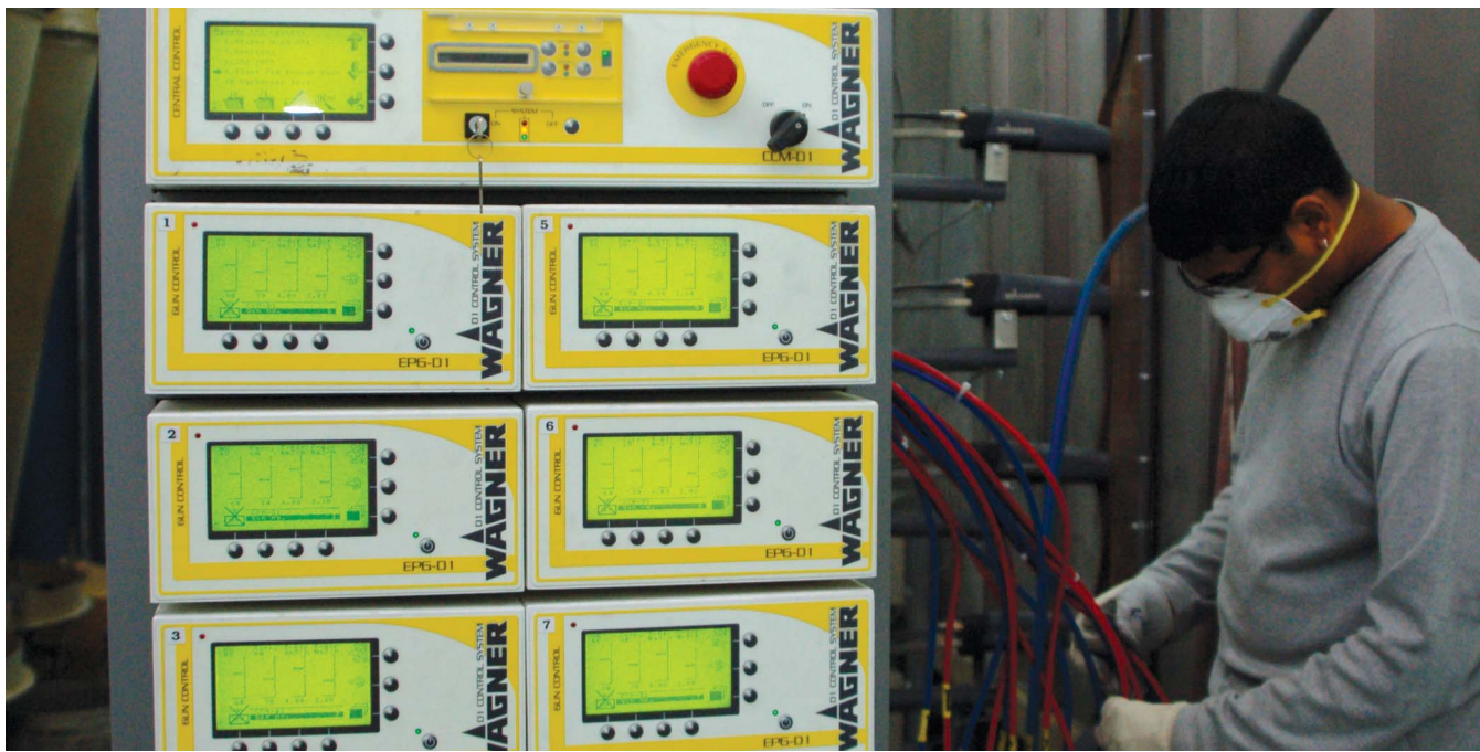
A Digitech computerized controller allows Colourific to precisely set and maintain the power delivery.
