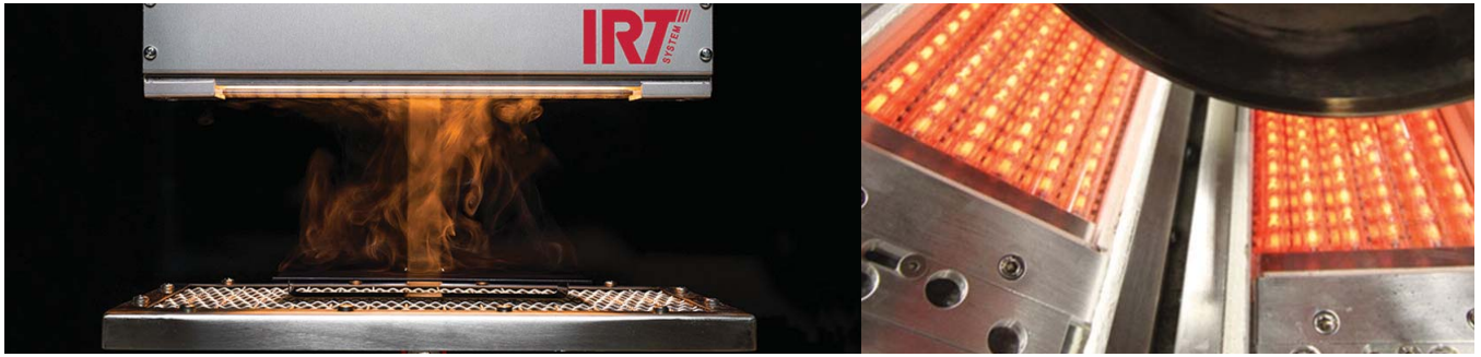
Heating units as used in Hedson's IR technology.
