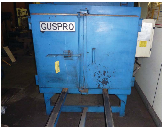
A long-serving Guspro pyrolysis oven.
