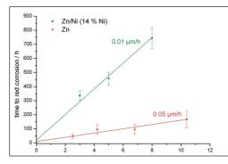
**Fig. 1:** Neutral salt spray test according to ISO 9227 for panels with increasing coating thickness of pure zinc (Protolux<sup>®</sup> 3000) and zinc-nickel (Reflectalloy<sup>®</sup> ZNA) leading in both cases to linear functions.
