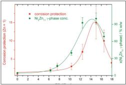
**Fig. 2:** Corrosion protection of zinc-nickel coatings with increasing nickel incorporation relative to pure zinc coatings (red dots) measured by neutral salt spray test (ISO 9227); Intensity of the (600) peak of the g-phase zinc-nickel alloy with increasing nickel incorporation (green dots) measured by X-ray diffraction
