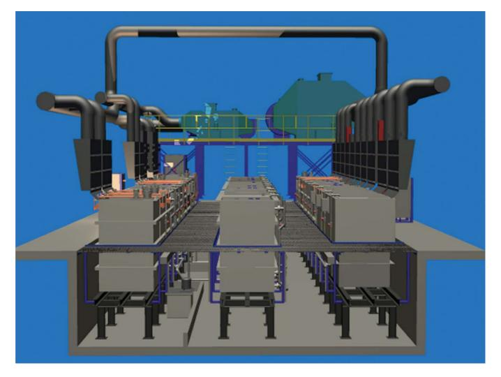
mated hoist systems use a monochrome touch screen with PLC that controls the hoist and all the safeguards associated with the hoist. The PLC follows a fixed timeway procedure through a series of travel, lift and drop commands. The time-way is a fixed sequence of moves that time after time will carry a flight bar through the process stations. There can be other peripheral control of hoist functions such as top sprays to rinse parts, mechanical agitation that starts and stops when the
