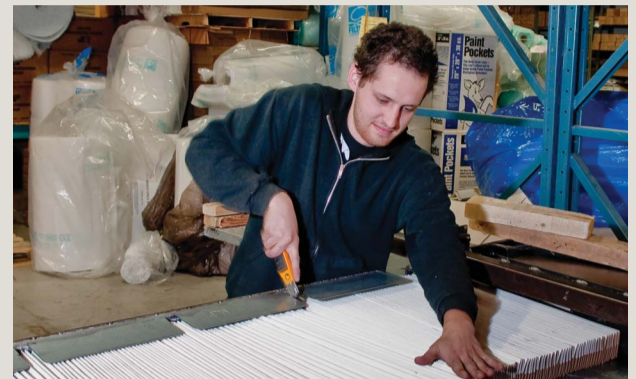
Tyler Paterson cuts the custom Servair pleated filter. The accordion style filter can also be cut to size by the end user.
