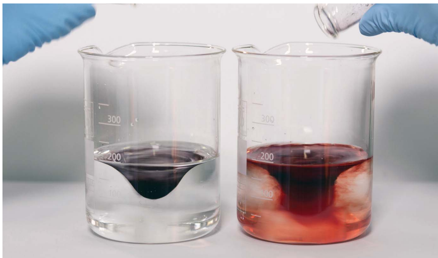
Landa pigments (right) disperse more easily in water than conventional types (left).
