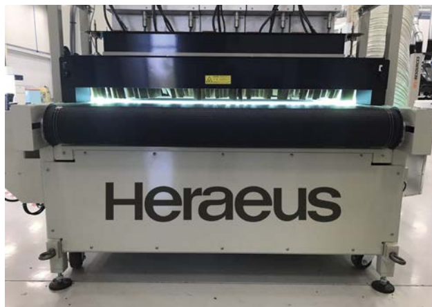
Flat line with 50-inch wide Heraeus microwave-powered UV curing system.
