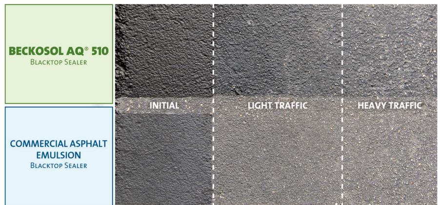
Composite photo showing results of a comparative study of Reichhold's Beckosol product and competing blacktop sealer.
