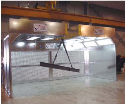
A part ready to be sprayed in a Crossing Air Spray booth.
