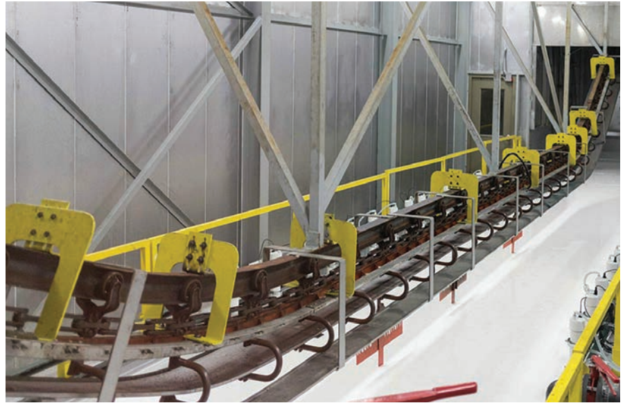
Koch E-coating conveyor system.
