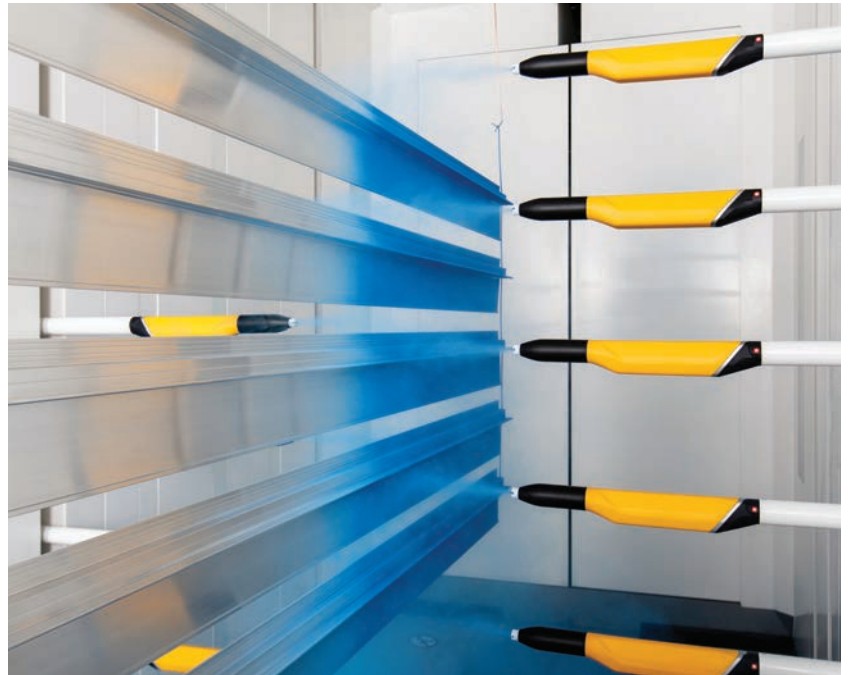
A powder coating line using Gema's OptiGun automatic spray units.
