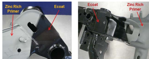
Zinc Rich Primer plus Epoxy Ecoat on welded underbody assembly.
