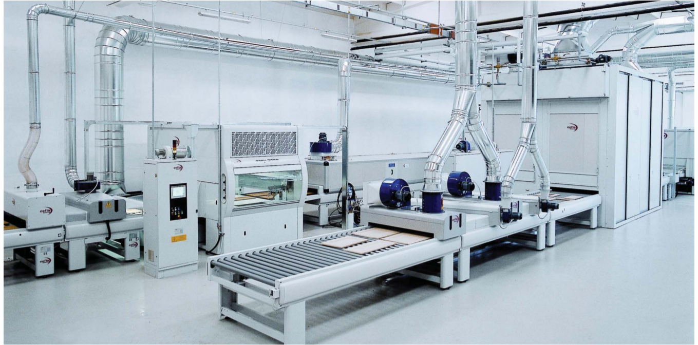
Fully automatic roll-coat and spray line for water-borne and water-borne UV coatings.
