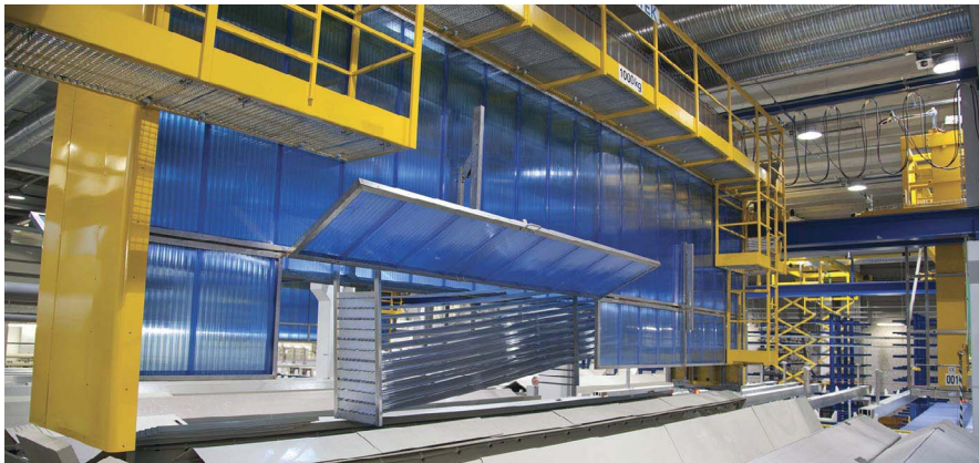
Galvatek automated anodizing line for extruded aluminum profiles. Plant includes ventilated transporters with tilting capability.
