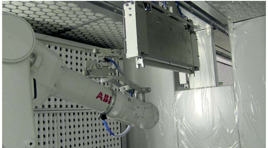
The carrier system is suitable for components of various sizes and shapes. The system offers high performance due to the parallel use of two linear axes.
