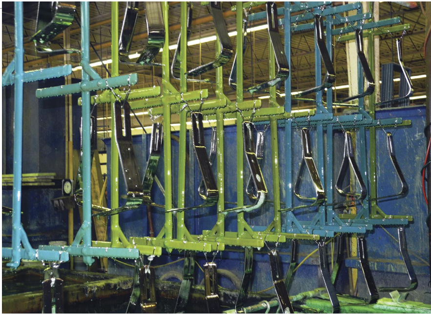
Racked decorative chair parts plated in a semi bright and a bright nickel.
