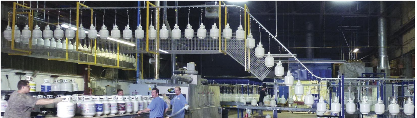
An enclosed track overhead conveyor for wet spray paint line from Pacline.
