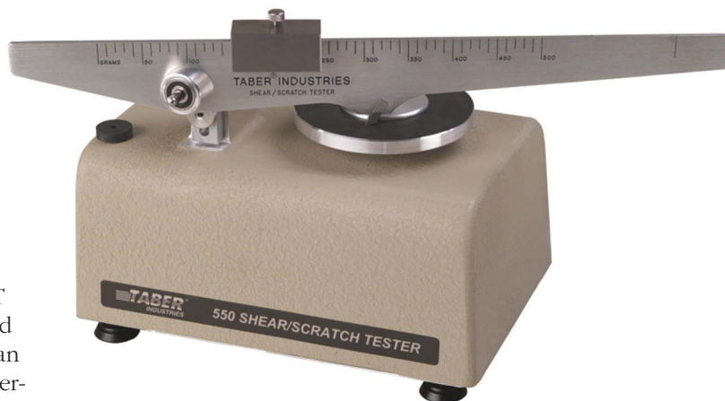
Taber's 550 Shear Scratch unit simulates what coatings undergo in daily use.
