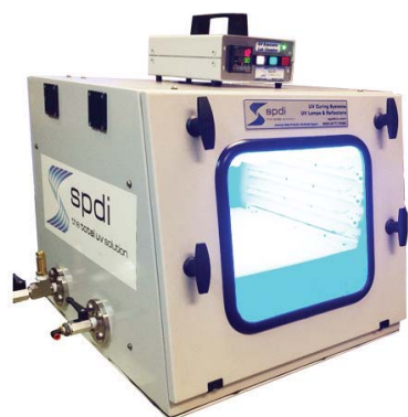
UV curing oven from SPDI (Delray Beach, FL).
