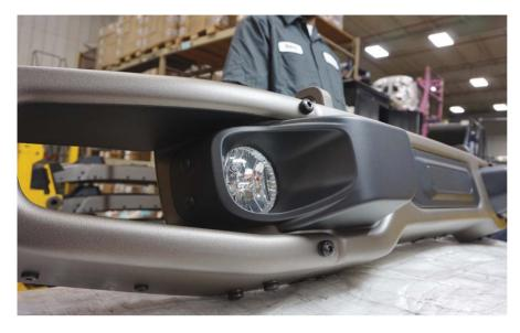
Powder coating on the front assembly of the Rubicon Jeep.
