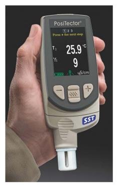
DeFelsko's new Bresle test unit, the PosiTector SST.
