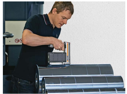
Fischer’s XAN-500 X-ray fluorescence instrument performs coating thickness measurement functions and other tasks. It can operate as a desktop unit or be integrated into production lines.
