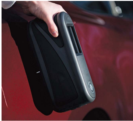
X-Rite MA-T unit measuring the gloss on a car's finish.
