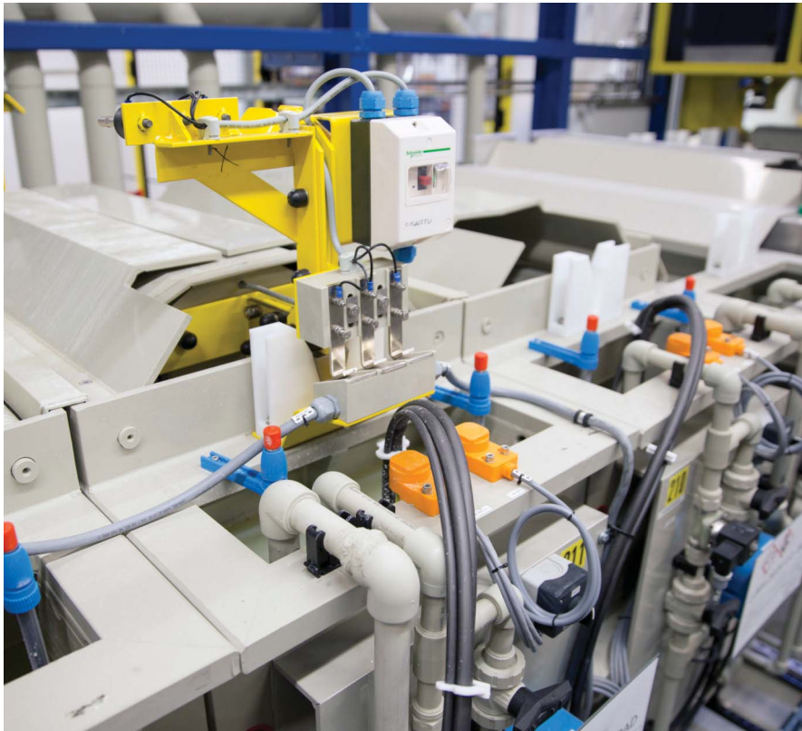
An automated electroplating line. Photo: Galvatek
