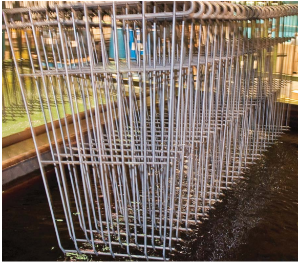
Shopping Cart lower trays being immersed into Zinc Phosphate post seal rinse.
