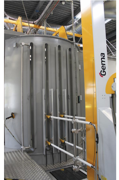
Left: MG 400 EH systems from SAMES KREMLIN are fitted with a fluidized powder tank. The powder pump is built into the gun and removable for cleaning. Right: Gema's MagicCylinder design ensures low powder accumulations and quick cleaning without entering the booth.
