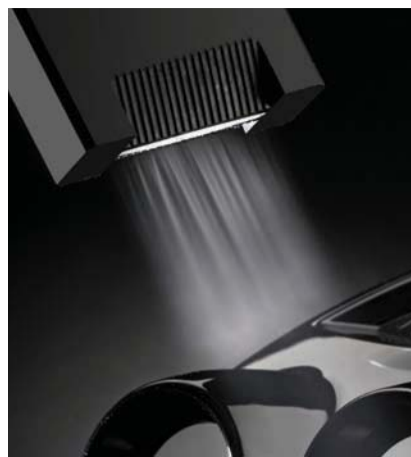
Particulates as well as film-like contamination can be gently removed from products made of various plastics and composites with CO2 snow-jet cleaning.
