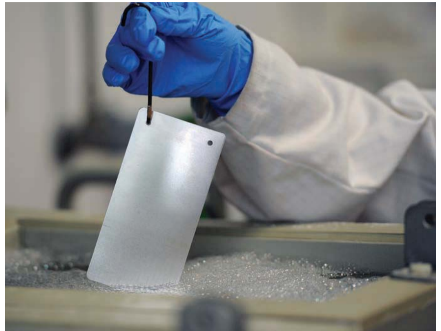
Degreasing with products based on renewable raw materials shows identically results compared to conventional degreasers.
