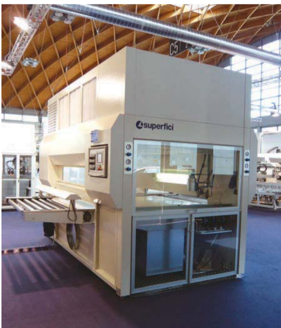
Superfici America, COMPACT PLUS/R Spraying machine with double arm reciprocator.
