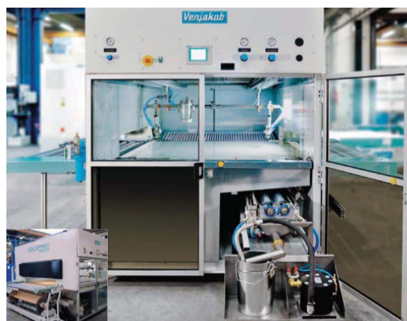
Superfici America, COMPACT PLUS/R Spraying machine with double arm reciprocator.
