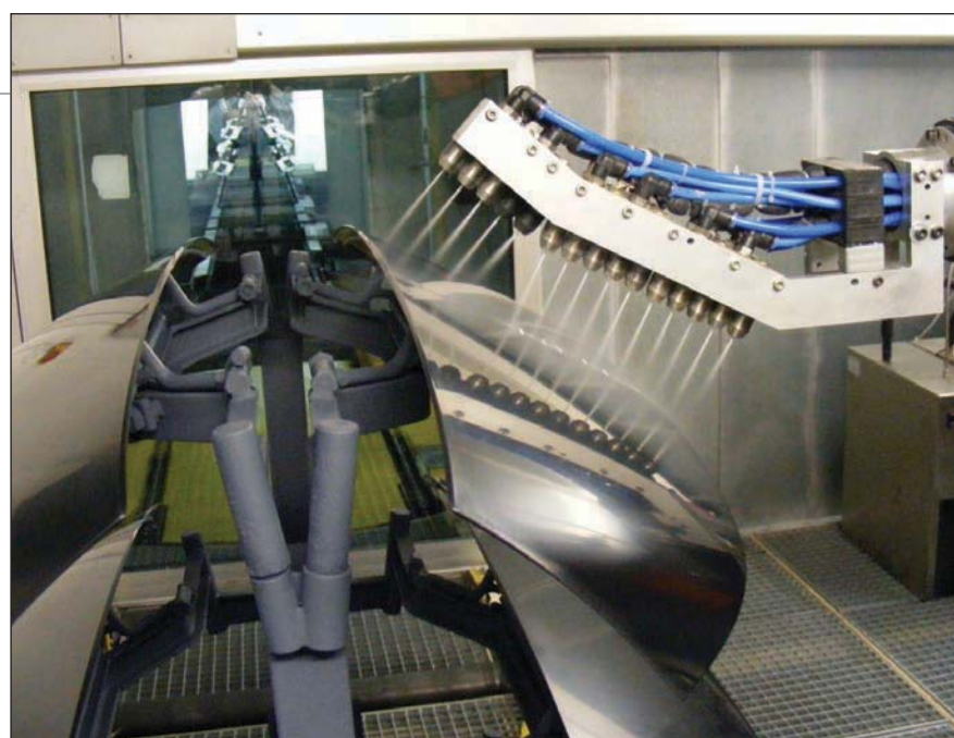
CO 2 snow-jet cleaning can be easily automated and integrated into the painting process.
