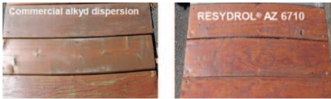
Wood coated with regular alkyd dispersion and sample with Resydrol AZ 6710.
