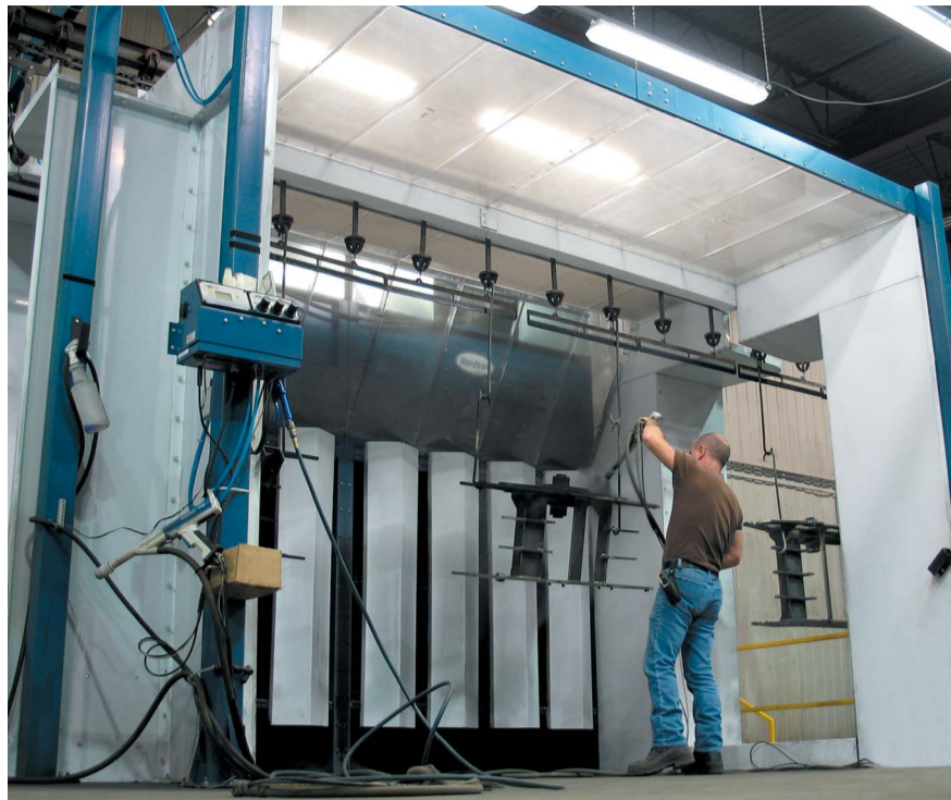
Manual spray booth Nordson Lean Cell, paint from Protech.
