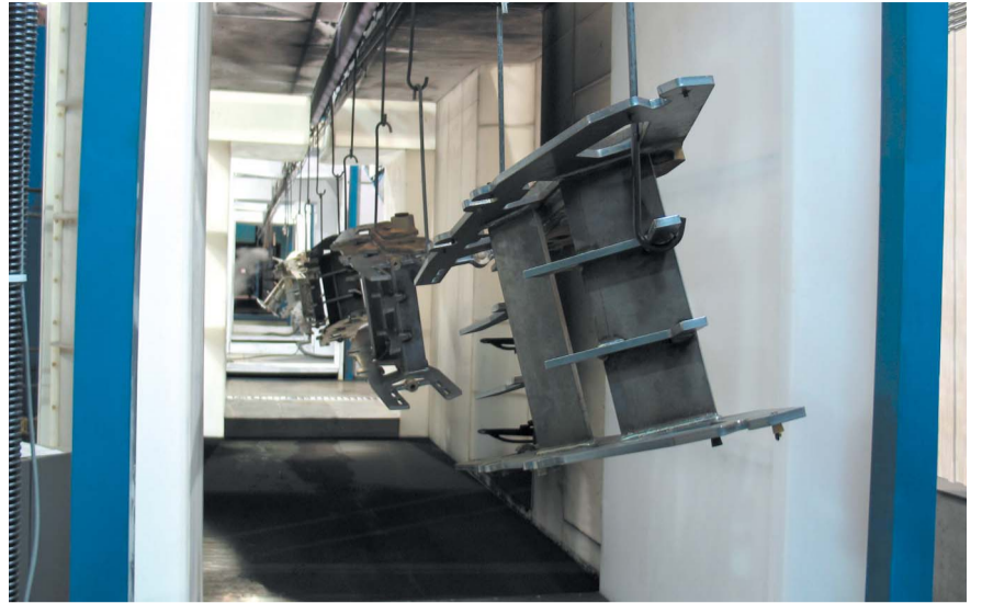
A part heading through Soucy's paint system on an overhead conveyor, automatic Nordson Excel 2001.
