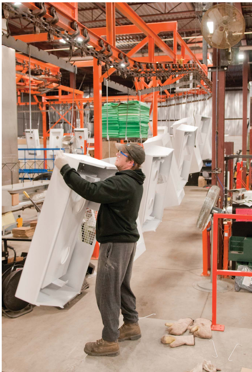
Andrew Howels offloads finished cabinet parts from the overhead conveyor.
