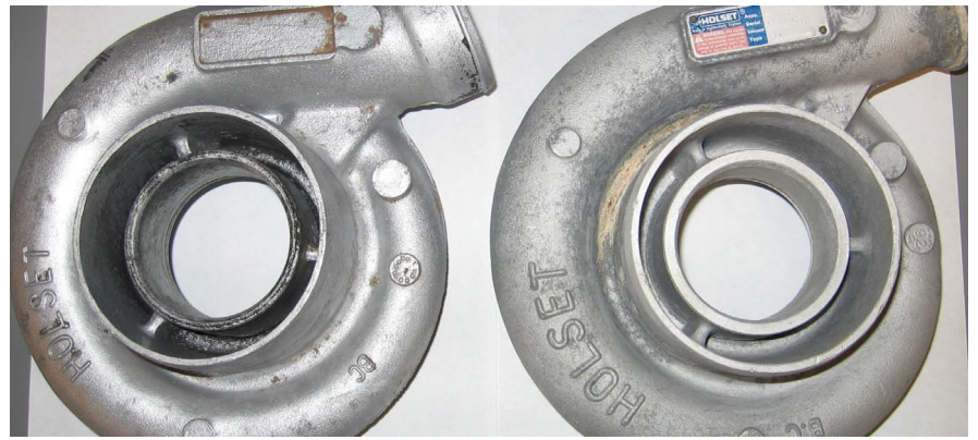
Parts After Paint Stripping. Photo supplied by Chemetall US, Inc.
