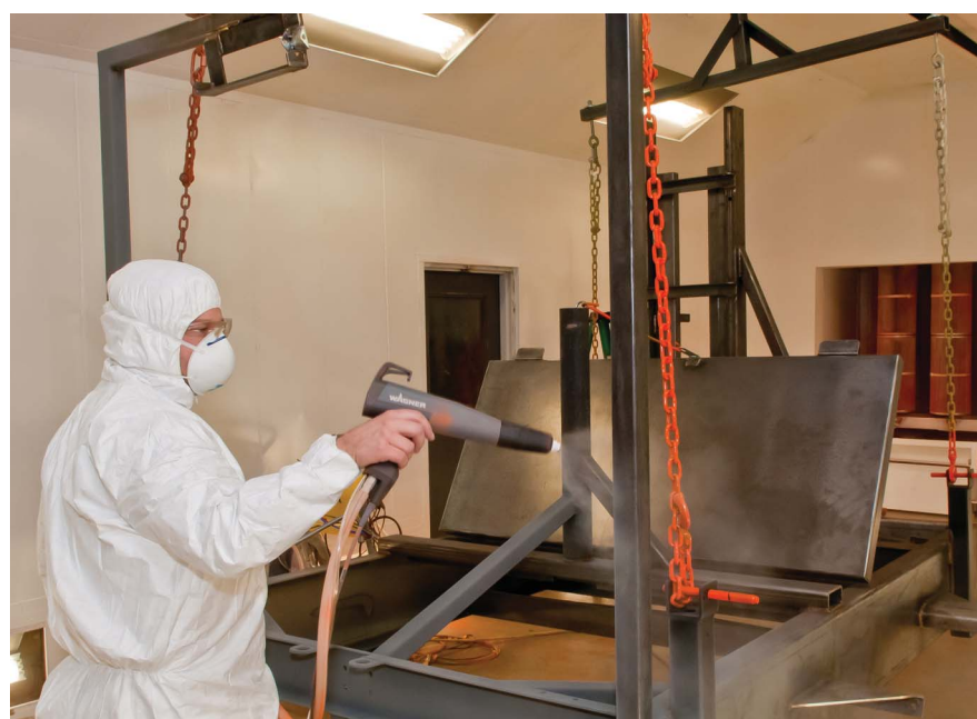
Doug Ker works in the custom built manual powder paint booth. He is working on a metal frame for a trailer used for traffic control in Germany.
