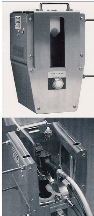
Chart 6: A gun flush box can be used with manual applicators to automate the colour change process.
