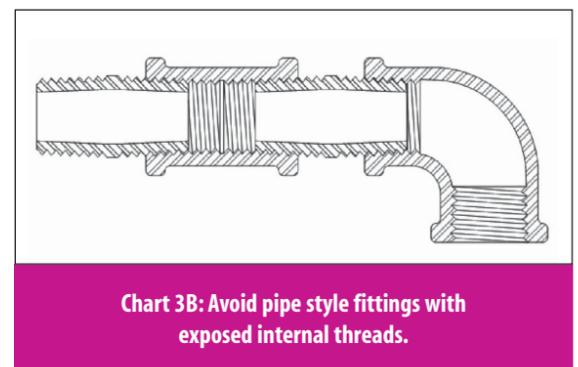
Chart 3B: Avoid pipe style fittings with exposed internal threads.
