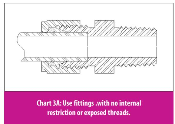
Chart 3A: Use fittings with no internal restriction or exposed threads.
