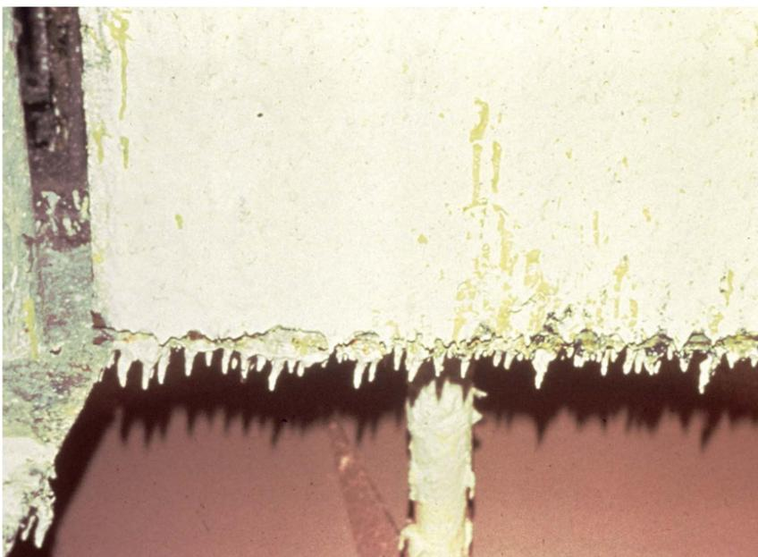
Semi-dried material left over from previous manufacturing batches provides an opportunity for the contamination of future batches.
