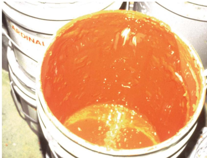
The number of transfer buckets must be kept at a minimum in the plant. Keep them clean (prepare a cleaning schedule) and protected from contamination.
