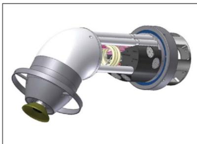
Chart 4: Some applicators have integrated fluid manifolds with dump and solvent flush valve.
