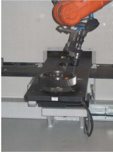
Time and cost savings are made possible through the use of selective cleaning of defined functional surfaces by means of CO2 snow jet cleaning, for example prior to laser welding.
