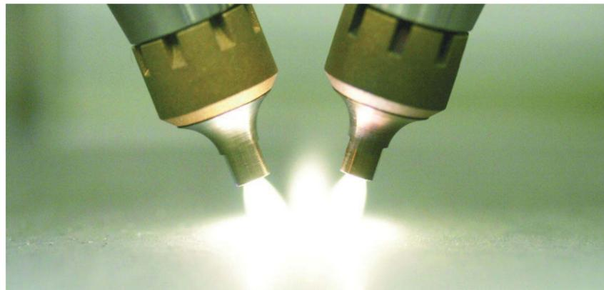
Plasma is suitable for fine cleaning and micro-cleaning of workpiece surfaces. Organic residues can be removed, and oxide layers on metal parts can be reduced as well. Further cleaning options include material removal by means of dry etching.
