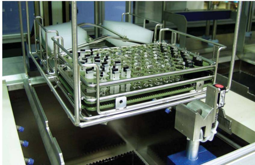
Parts in the cleaning basket made of round wire are well rinsed on all sides by the cleaning medium. In addition to this, wire basket systems are distinguished by good draining characteristics which minimise cleaning agent and contamination carryover.
