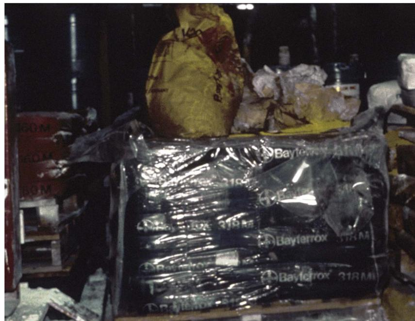
Open bags and partially used bags should be protected from contamination. Litter has to go!
