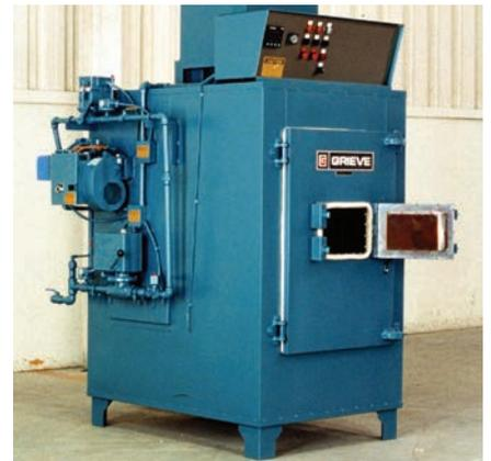
No. 915 is a gas-fired, 650-deg F cabinet oven from Grieve, currently used for testing paint coupons. Workspace dimensions measure 26x26x38 in. The modulating gas burner has 100,000 BTU/hr installed, while a 1000 CFM, 1-HP recirculating blower provides vertical upward airflow to the workload.
